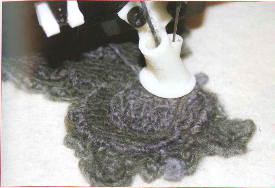
A 3-D printer developed by Carnegie Mellon University and Disney Research Pittsburgh feeds yarn into desired shapes and uses a needle to turn the yarn into a loose felt fabric object.
