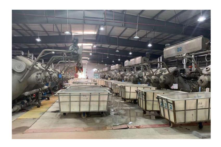
The dyeing factory has 23 sets of dyeing overflow tanks, 7 sets of molding machines and 10 sets of finishing machines, which can process polyester ammonia, nylon ammonia and blended fabrics.
