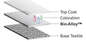
Combination of bio-content and recycled inputs to create material system suitable for specific performance and end-use.
